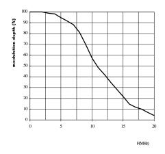
Fig. 2 Typical square-wave response curve.
